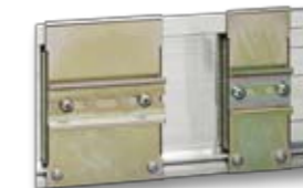
SLZ10 ... SLZ14 Mounting bracket for the S7-300 rail Bracket: Width of unit: SLZ10 up to 40mm SLZ11 41 to 51mm SLZ12 52 to 66mm SLZ13 67 to 90mm SLZ14 91 to 121mm
